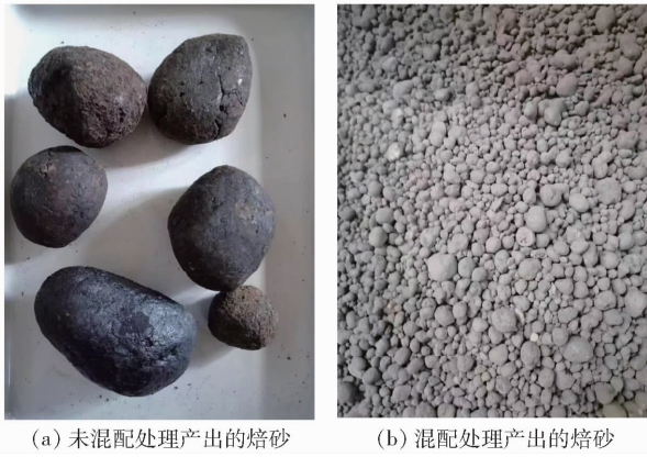
图 6 铜阳极泥混配前后硫酸化焙烧后渣形貌 Fig.6 Morphology of slag after sulfating roasting of copper anode slime before and after mixing
